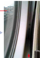
客室窓枠 [吸音材・隙間埋め材 (難燃性)] Passenger-car window frames [sound-absorbing material, material for filling clearances (fire-retarding)]
